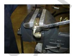
Now thread the fitting into the shell clockwise. You do not need to bottom out the fitting. You can leave a couple of threads showing. If install 90 degree fittings on both ends of the hose you will find that you will probably have to clock the fittings.
