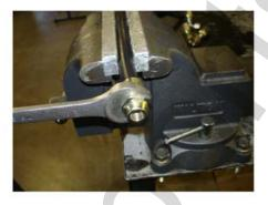
Next thread the shell onto the hose counter clockwise until the hose bottoms out in the fitting.
