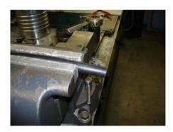
First you need to determine the length of hose required and cut to length. We suggest using a abrasive cut off wheel. Then clamp hose in vise with about 1.5" protruding out.
