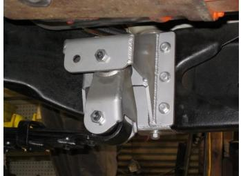
When using stock rear springs from a '73-87 ½ ton Chevy you will be using the rear shackle bolt hole in these brackets
