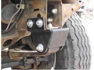
Position rear hanger such that the distance from the main eye centerline to the upper shackle bolt is 51". You will be using the rearward most shackle bolt
