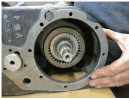
Install the input bearing, the outer snap ring and the snap ring that holds the bearing to the shaft. Re-assemble the rear output assembly of the NP205 just as it was removed.
