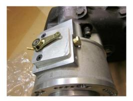
You can fill the Magnum box from either the shifter housing opening or the fill plug location, capacity is 1-1/2 pints (or ¾ of a quart) of automatic transmission fluid or gear oil (80W-90 etc). To visually inspect fluid level, install a clear vinyl sight tube between a barb fitting in the drain hole and a "T" fitting in the vent location or a barb fitting in the fill hole.
