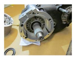
The front half of the Magnum system is pre-assembled at Offroad Design. If you need to disassemble these parts, the procedure is essentially the same as any of the 23X/24X/26X/27X series of New Process transfer cases.
