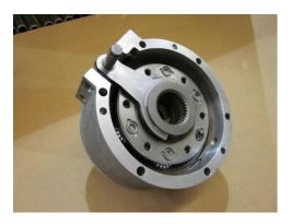
Install the front half of the Magnum to the rear housing, making sure that the shift hub, shift fork and shift rail all stay with the front case half. Apply a light coating of silicone sealant (we use "The Right Stuff") to the face of the case half to seal the case interface.
