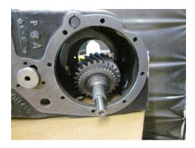
Install the clutch ring onto the shift fork, the shift rail may need to be manipulated for clearance.
