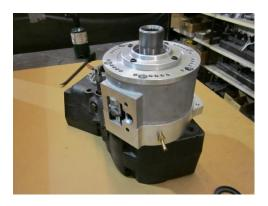
Install the shifter housing using the two supplied bolts, seal the shifter housing with silicone sealant.
