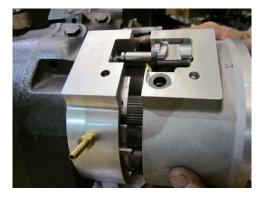
Apply blue Loctite to the long socket head cap screws and install them to fasten the two case halves together, torque to 40 ft. lbs.
