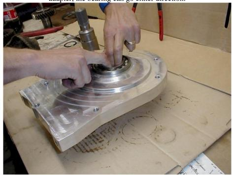
13. Install the original snap ring into Doubler adapter.
