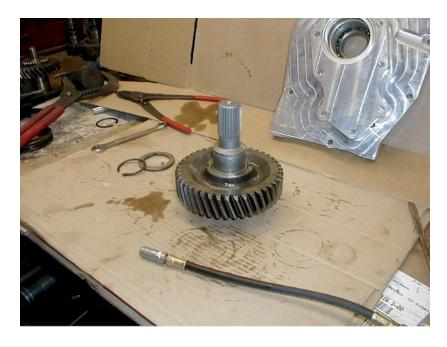
17. Install retaining pin if you'd like (it keeps the thrust washer from spinning but that doesn't really accomplish anything, so don't feel bad if you lost it) and install thrust washer over the Doubler shaft.
