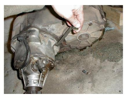
3. Lift the housing off the chain case, a little persuasion from a hammer may be needed but the two should come apart fairly easy.
