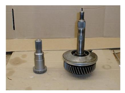
9. Remove the snap ring that holds the gear/retainer on the shaft, this is where you'll need the big snap ring pliers.
