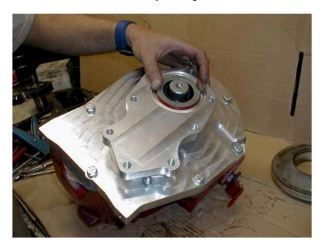
22. Install the 15 fat needle bearings into the pocket in the Doubler shaft, use grease to hold the needles in place.
