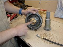
16. Place low gear on Doubler shaft, note that the clutch teeth are face down, next to the clutch teeth on the Doubler shaft.
