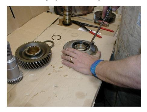
12. Remove the bearing from the original retainer and install it into the Doubler adapter, the bearing can go either direction.
