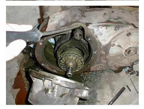
5. The next step is to remove all the bolts holding the chain case to the range box.
