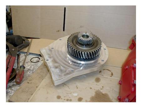
21. <u>If you're using a GM/Dodge figure 8 style NP205:</u> Install seal into Doubler adapter, the spring goes towards the NP203. Seal must be 1/2" below <u>gasket</u> surface and no more than 5/8", be careful not to damage seal.
