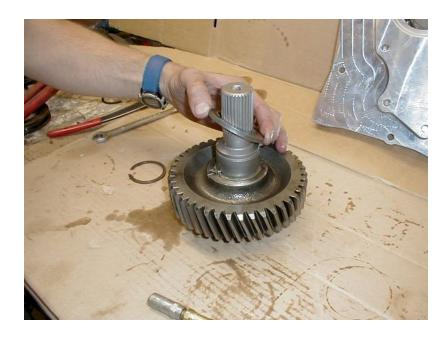
18. Install doubler adapter over shaft assembly. You may need to heat up the bearing, this is a precise fit.
