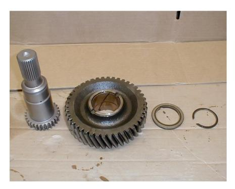
11. Remove the snap ring that holds the bearing into the retainer
