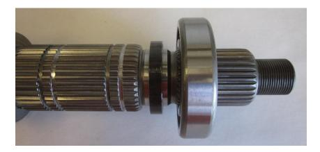
Install the seal into the bearing/seal retainer, a touch of RTV silicone on the OD of the seal can help if there are any minor imperfections. Remember to oil both the seal ID and yoke OD before final assembly.
