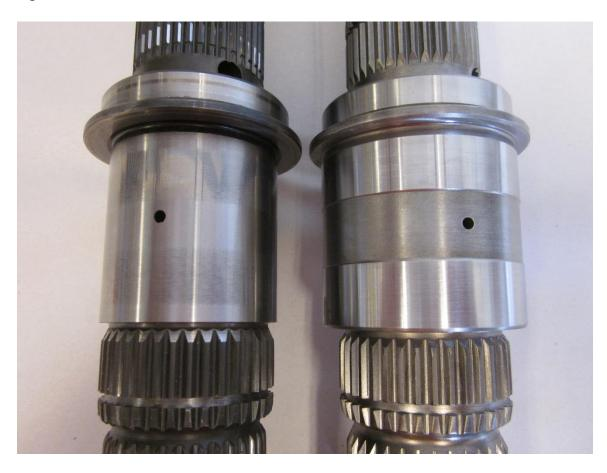
The depth on the pump seal is important. This seal below has been driven beyond flush and can cause problems:
