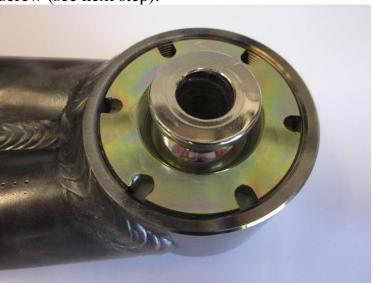
g. Apply thread locker to set screw and install it so that the adjuster nut is locked in place
