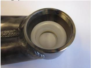
d. Install ball, it's symmetric so it can be installed either way
