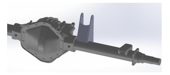
Your truck naturally wants to twist towards the passenger side under torque, basically your springs are resisting the torque running through the driveshaft and because your engine rotates clockwise, that makes the truck lean to the passenger side under torque. Your traction bar will actually try to lift up the corner of the vehicle that it's installed on as it resists the torque running through the axle tubes.
