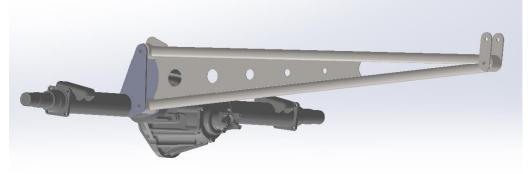
Example of traction bar installation on a truck with moderate or no lift, the traction bar is nearly level with the ground and the shackle is pointing down.
