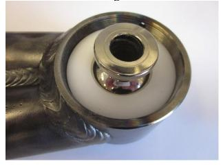
f. Install threaded adjuster nut with the logo out. While a spanner wrench is the right tool here, a punch and hammer work just as good to tighten this nut. Snug is good here, make sure that one of the slots in the nut line up with the threaded hole for the set screw (see next step).
