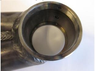
b. Place washer into flex joint housing
