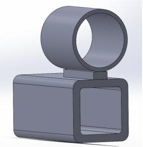
Once that's fully welded, the two thinner plates are welded between the crossmember and tube as pictured
