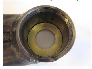
c. Place bushing half into flex joint housing, both bushing halves are identical. Make sure the concave side of the bushing is facing up.
